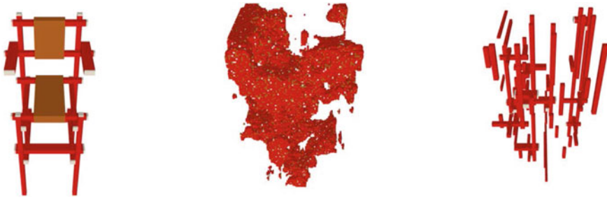
Fig. 18 (LEFT) Reconstructed model of Gerrit Rietveld’s Baby Chair encoded as voxels. (MIDDLE) Initial input massing via perlin noise generation. (RIGHT) Generated output that failed to capture the planar features of the original input model and its function as a chair
