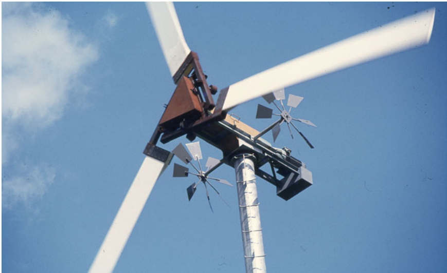
Fig. 27 The early passively controlled wind turbine from Lagerwey van de Loenhorst with variable speed. Diameter: 10 m. Photo Jos Beurskens
