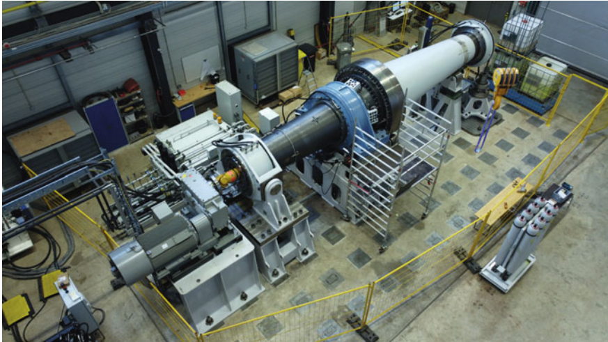
Fig. 9 Experimental setup at Fraunhofer IWES to investigate the fatigue strength of a cast shaft [Fraunhofer IWES]
