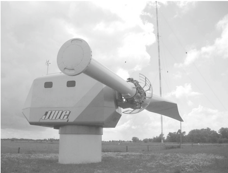
Fig. 7 One-bladed wind turbine monopteros on the DEWI-test field near Wilhelmshaven. Photo Alois Schffarczyk
