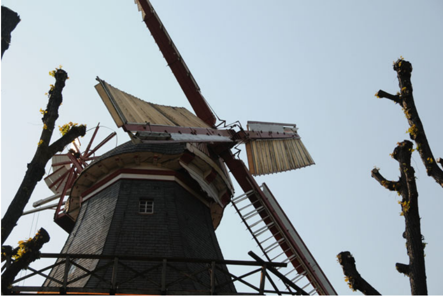
Fig. 10 Louvre blades of the mill on the Wall in the centre of Bremen. Photo Jos Beurskens
