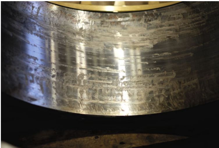
Fig. 10 Traces of bearing creep on contact surface to the bearing seat of a main bearing inner ring [Fraunhofer IWES]
