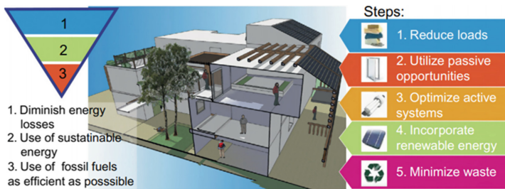
Fig. 6. The fundamentals of the ZEB project.
