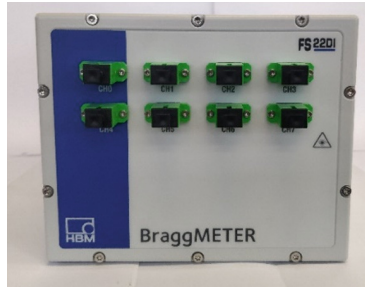
Fig. 6. Interrogator FS22 Industrial BraggMETER used in the laboratory work.
