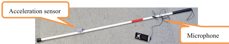
Fig. 4. Modified white cane with sensors.
