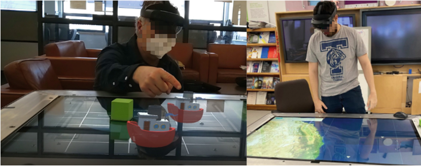
Fig. 3. Users are interacting with the SD wearing HoloLens. The HoloLens first-person vision of augmented reality interaction over the SD at the left. A third person of the user interacting with both systems is on the right.
