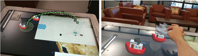
Fig. 4. The user selects a piece of vessel information (the user can grab and drag a the AR object to use this element to get more details about the selected vessel).
