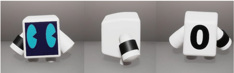
Fig. 2. Final design of the robot from three perspectives (front, side, back).
