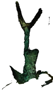
Fig. 6. An approximated surface mesh obtained by AlphaShape. Image captured by Meshlab application.
