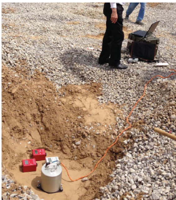
Fig. 8 Seismic test for stone column test area
