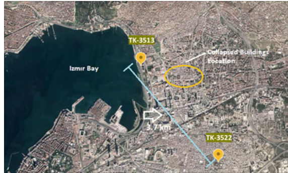
Fig. 1 The map showing the strong ground motion stations and the site of collapsed buildings location
