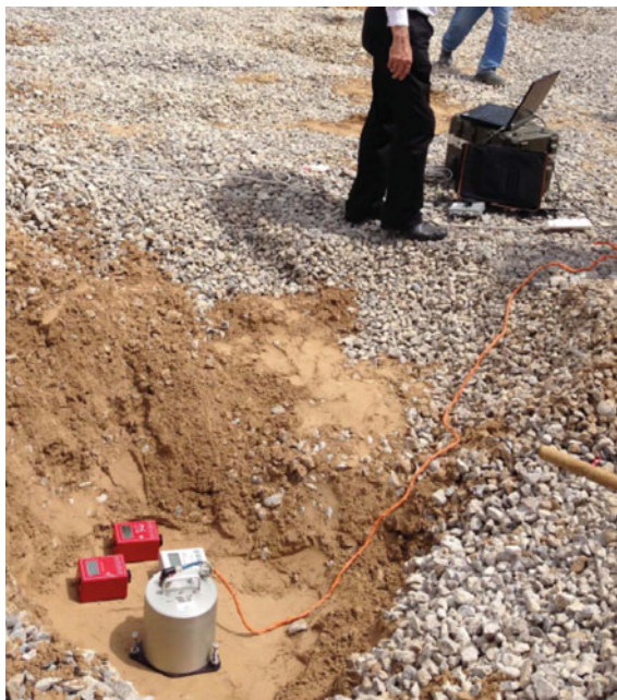
Fig. 8 Seismic test for stone column test area
