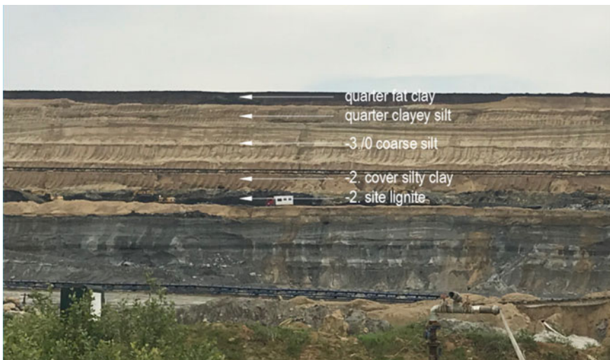
Fig. 1 Soil layers of the border slope in Eastern no. III. mine, Visonta
