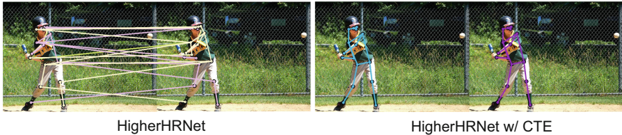
Fig. 5. Effectiveness of CTE in human pose estimation. Here we apply an extreme case – copy-and-paste the same object. HigherHRNet with CTE (right column) can distinguish local responses with similar visual appearances in different locations, making the pull-push grouping more reasonable, while the original HigherHRNet failed.
