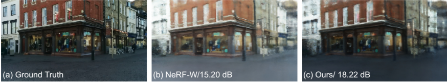
Fig. 4. Typically NeRF only renders views that reflect the appearance of its training sequences, as shown by NeRF-W’s synthetic view (b). However, in relocalization tasks, the query set may have different appearances or exposures to the train set. The proposed histogram-assisted NeRF (c) can render a more accurate appearance to the unseen query set (a) in both quantitative (PSNR) and visual comparisons. We refer to the supplementary for more examples.
