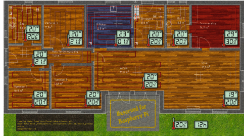
Fig. 3. Digital twin of a floor heating system
