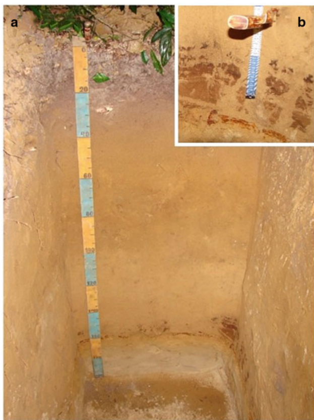
Fig. 14.20 Arenosol on a Pleistocene marine terrace under Tall Restinga Forest (Bertioga, São Paulo state), formed from the degradation of an originally poorly drained Podzol, the drainage of which improved due to the accelerated lowering of the water table. a Detail of the lower part of the profile with relics of the old Bh and the placic horizon, both in advanced degradation b Photo: Mauricio R. Coelho
