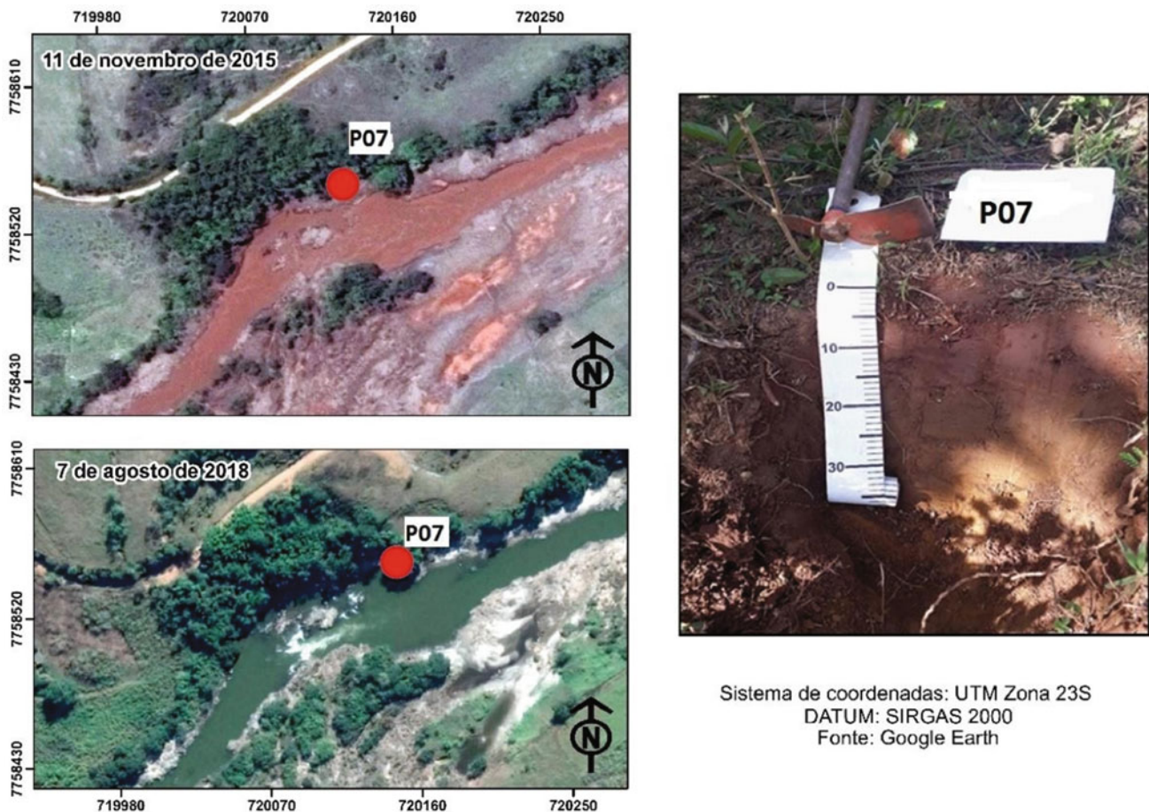
Fig. 17.15 Technosol site 7 before and after the disaster and the soil profile collected. Collection point number 07 is downstream of the Doce River. A 15 cm layer of tailings was observed, followed by the C horizon of Neossolo Flúvico. It was also observed the presence of thin
