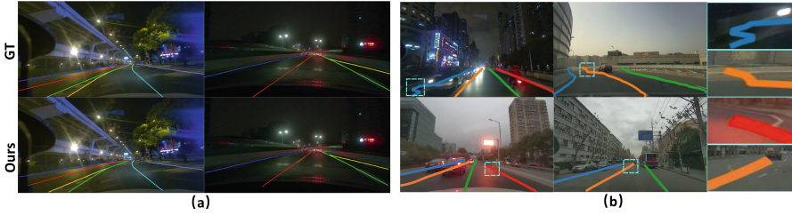
Fig. 1. Challenging scenes (curve lanes, Y-shape lanes). The first row of (a) shows the ground truth while the second row is our predictions. The first row of (b) shows the result of segmentation-based methods that global shape of lane is not well fitted. While the second row of (b) shows proposal-based methods, can not depict local locations of Y-shape and curve lanes.
