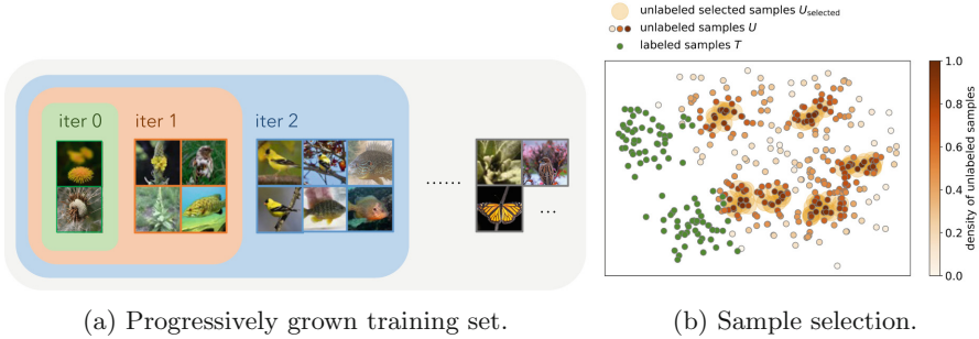
Fig. 1. Progressive Sample Selection (PSS) approach. (a) shows the progressively grown training set. The training set gradually expands during iterations. (b) shows a toy example of sample selection in one iteration. We select samples that are densely clustered together with high local homogeneity
