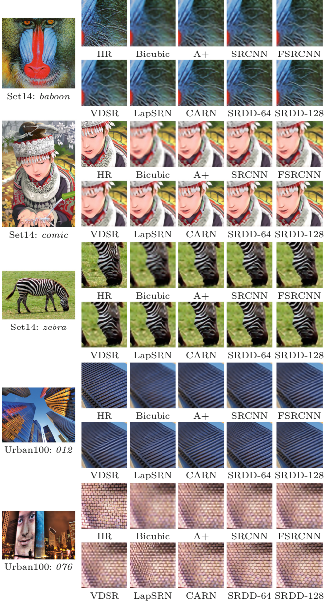
Fig. 8. Visual comparison for \times 4 SR on Set14 and Urban100 dataset. Zoom in for a better view.
