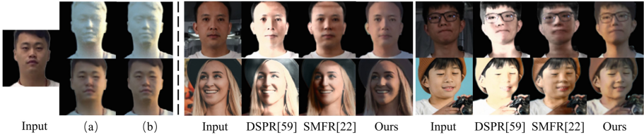
Fig. 8. Left: Ablation of face refinement module. (a) Top: cropped face from the refined full-body shading map Bottom: corresponding relit result (b) Top: refined face shading map Bottom: corresponding relit result. Right: Comparison with existing portrait relighting methods.
