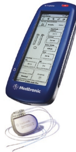
Fig. 44.1 Medtronic ENTERRA II device, two electrodes, and N'Vision Clinician Programmer
