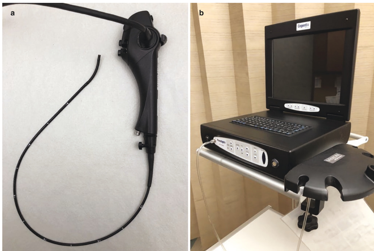
Fig. 22.1 Transnasal endoscopy. (a) PrimeSight TNE-5000 transnasal flexible esophagoscope (length 650 mm, field of view 110°, outer diameter of EndoSheath protective barrier (not shown) 1.5 mm or 2.1 mm.
