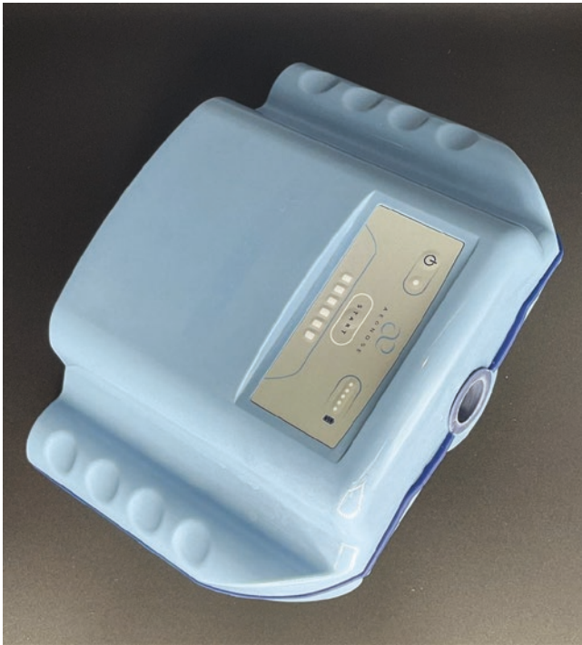
Fig. 22.6 Electronic nose device. The Aeonose is a handheld device that consists of an array of metal oxide sensors, which when in contact with volatile organic compounds (VOC) produce a unique signal representative of the VOC composition of a breath sample. To generate a VOC signal, a patient breathes into a mouthpiece for several minutes
