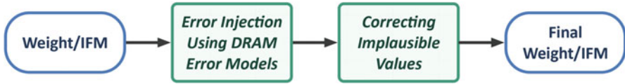
Fig. 6 Methodology to incorporate DRAM error models in the DNN evaluation framework. Adapted from [23]
