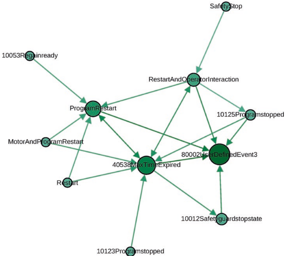
■ Fig. 9.12 Example graph (Atzmueller et al., 2019a) with respect to the event “80002:UserDefinedEvent3.” The graph is compiled from the respective sequential log data, i.e., preceding and consecutive events. Then, given a specific event, all paths to this event can be analyzed in more detail. We refer to Atzmueller et al. (2019a) for a detailed discussion
