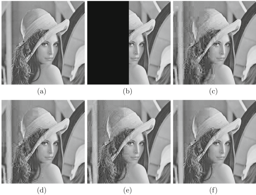
Fig. 7. Reconstruction results comparison for an aggressive attack in Lena image. (a) Original image. (b) Tampered image. (c) Reconstructed image [13]. (d) Reconstructed image [21] with T_d = 50 . (e) Reconstructed image OMP+VDSR with T_d = 0 and (f) Reconstructed image OMP+VDSR with T_d = 42 .
