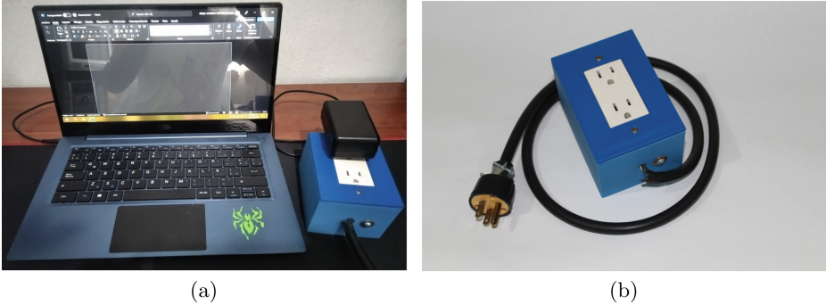
Fig. 2. IoT Device for energy consumption monitoring. a) Figure on left side presents the IoT device operating with a computer laptop. b) Figure on right side presents the IoT device used in this paper.
