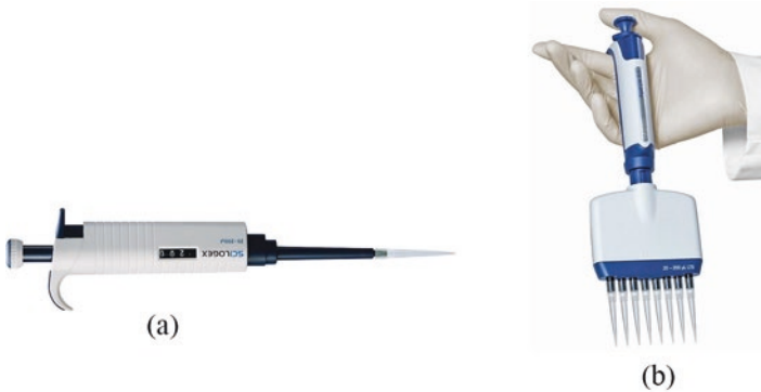
Fig. 2.7 Pipettors: (a) variable-volume pipetting device, (b) Multipoint pipettor with manifold for 8 plastic tips; 4 and 12 are also available https://www.scilogex.com/micropipette-single-channel-fixed-pipettors.html , https://www.mt.com/in/en/home/products/pipettes/manual-pipettes/multichannel-pipettes.html
