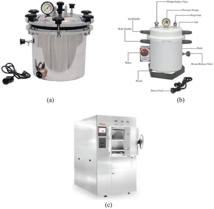
Fig. 2.35 Autoclave: (a) small laboratory autoclave, (b) labelled laboratory autoclave, (c) large laboratory autoclave
