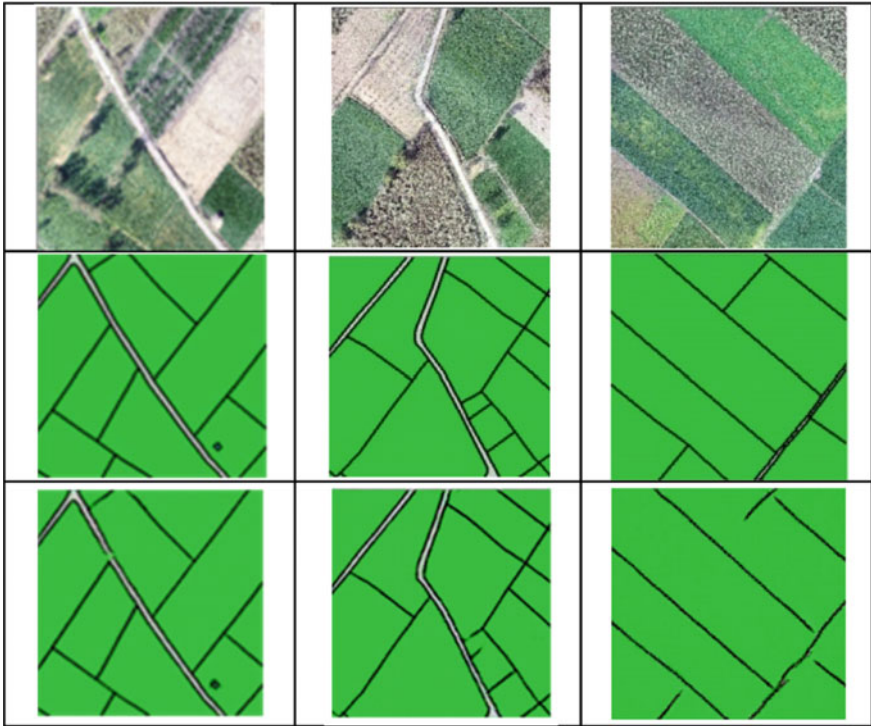
Fig. 4 The generated output with the image-to-image translation model during training. The source UAV image (top), the ground truth (in the middle), and the predicted image during training (bottom)
