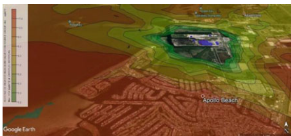
Fig. 39 24 h NO x dispersion from the TECO Big Bend power plant in Tampa Florida
