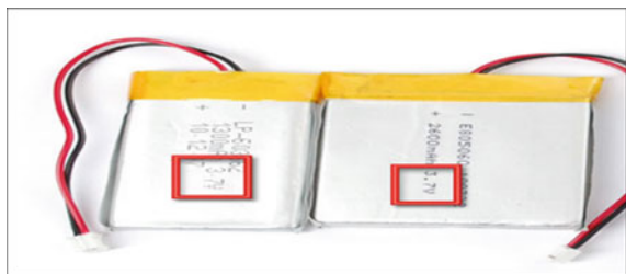
Fig. 1 LiPo battery showing nominal voltage (3.7 V). Courtesy https://learn.adafruit.com/assets/979
