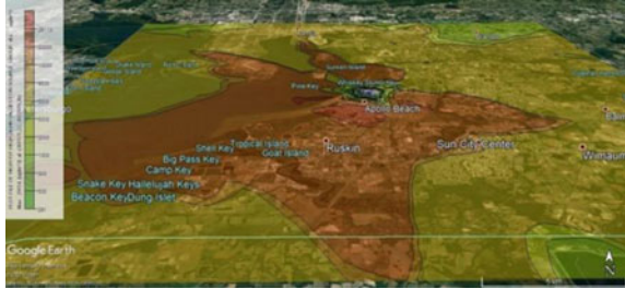
Fig. 36 24 h CO 2 dispersion from the TECO Big Bend power plant in Tampa Florida
