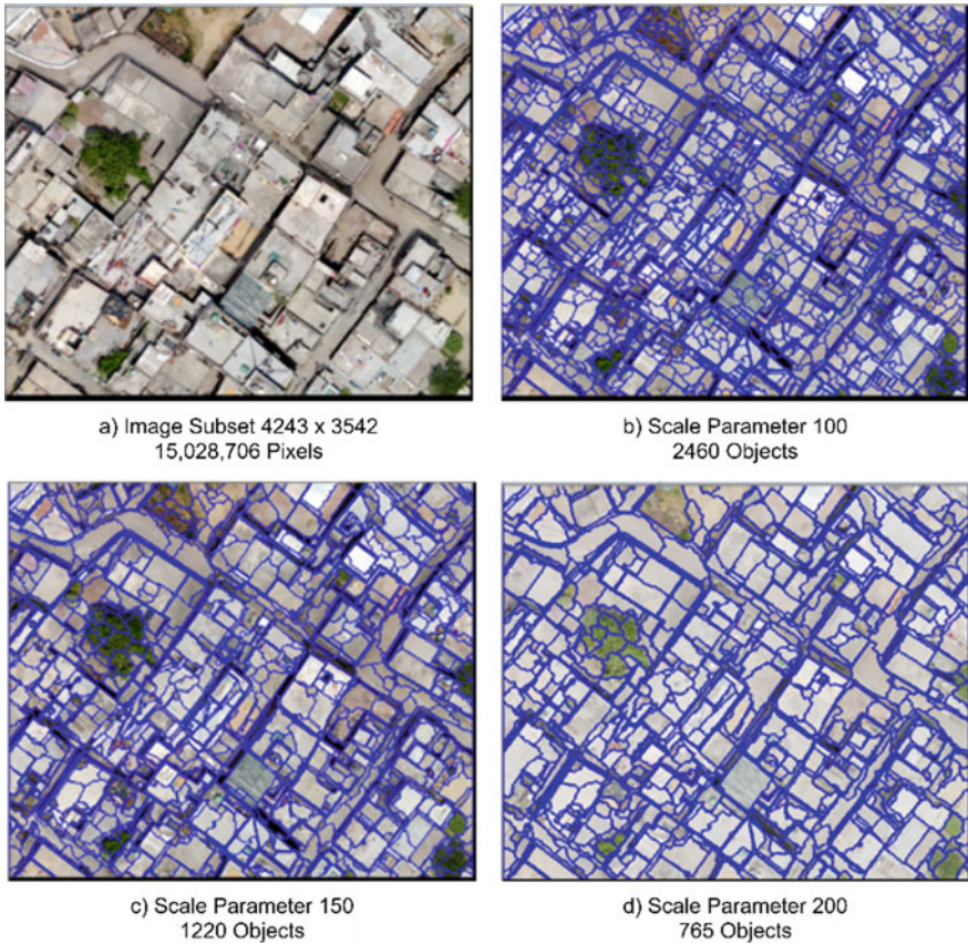
Fig. 6 MRS segmentation using different object primitives and resulting image objects
