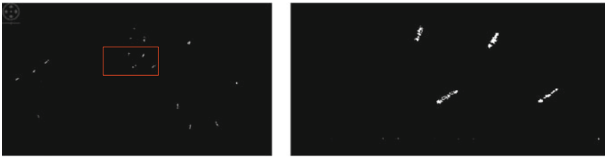
Fig. 11 CFAR results are shown for T_{11} where a represents the area near coastline and b represents the zoomed area in the red box
