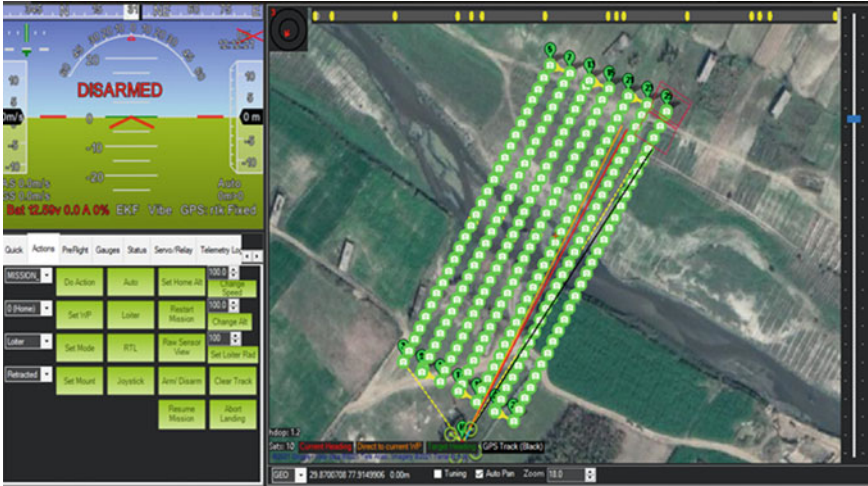
Fig. 4 Flight plan of the area in mission planner
