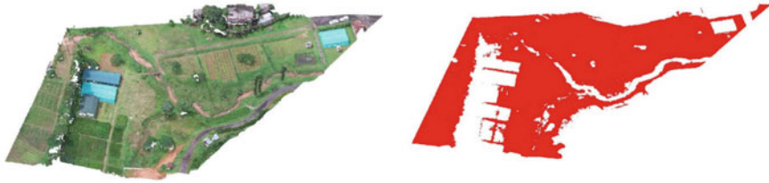
Fig. 4 Planar ground points segmentation (right) from source point cloud (left) using RANSAC
