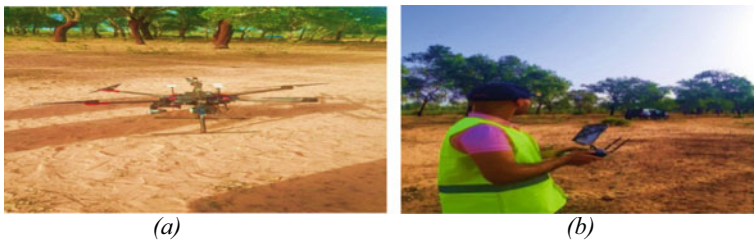
Fig. 4 a DJI M600 pro drone used for the first point cloud. b Photo of the first mission
