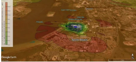
Fig. 42 1 h SO 2 dispersion from the TECO Big Bend power plant in Tampa Florida
