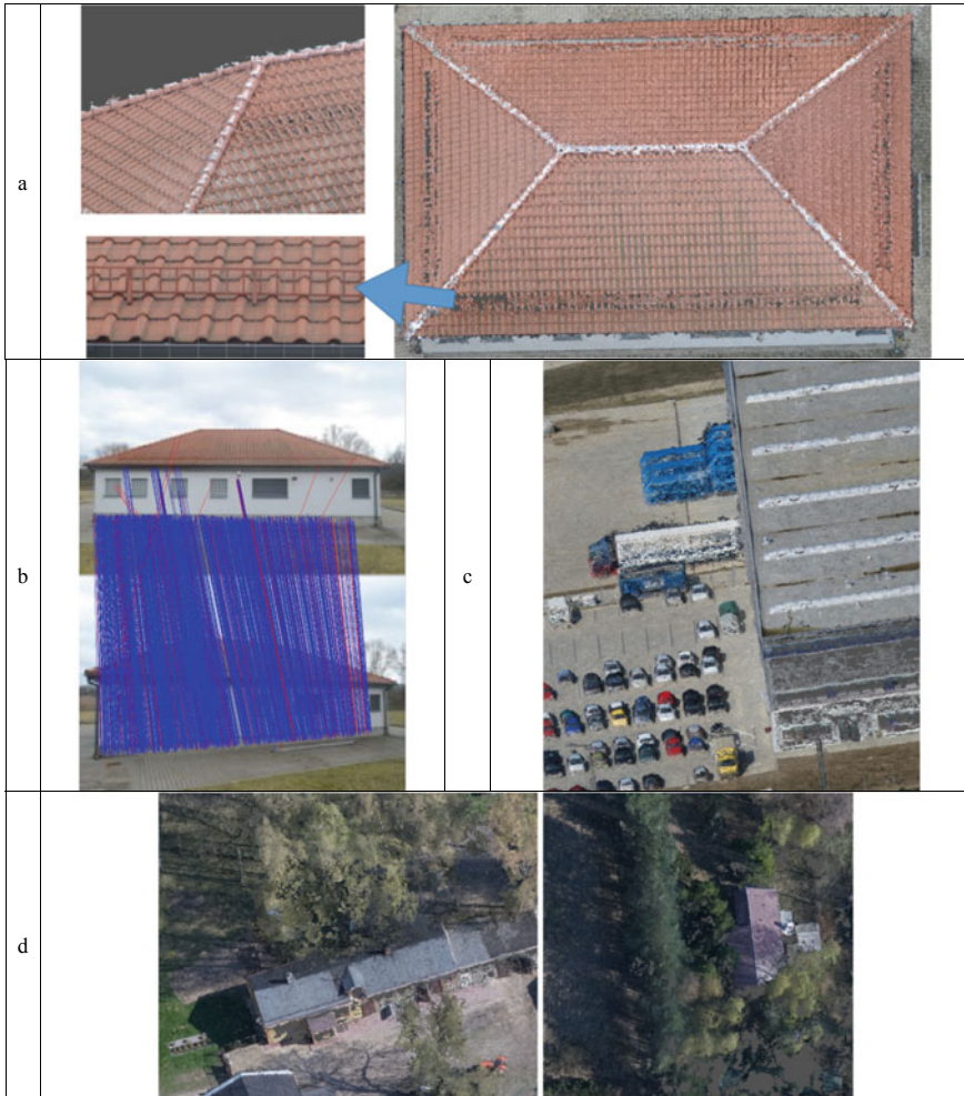
Fig. 2 Visualization of issues related to different measuring techniques. a Lack of details on roofs and noise using TLS or terrestrial imagery, b The issue related to tie point localization on building façade with homogenous structure, c The lack of façades consistency or reconstruction errors when using only nadir images, d The issue related to buildings partially occluded by vegetation—mainly occur in airborne imagery
