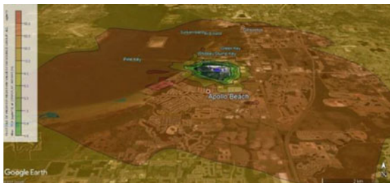
Fig. 38 1 h NO x dispersion from the TECO Big Bend power plant in Tampa Florida
