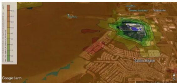
Fig. 37 1 h NO x dispersion from the TECO Big Bend power plant in Tampa Florida
