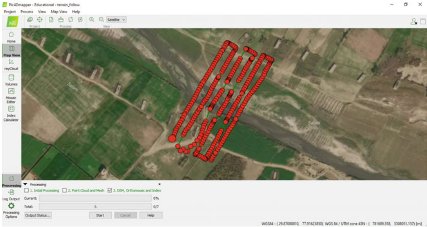
Fig. 6 Data processing in Pix4D
