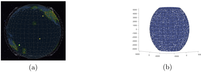
Fig. 2. Starlink constellation vs our model. (a) Starlink constellation of 2806 satellites; (source: https://satellitemap.space/?constellation=starlink ) (b) 2806 random points uniformly distributed on the surface of sphere.
