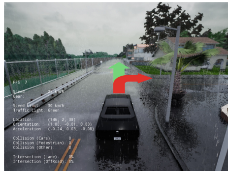
Fig. 2. An example of navigation command failure. The navigation command given at the intersection is Go Straight (as shown by the green arrow in the figure), but the motion controls output by the driving policy model make the vehicle turn right at the intersection (as shown by the red arrow in the figure). (Color figure online)
