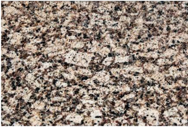
Fig. 17 Thunder Stone granite. Size of a large crystal 1.3 sm. Photo by Georgy Popov, 2016
