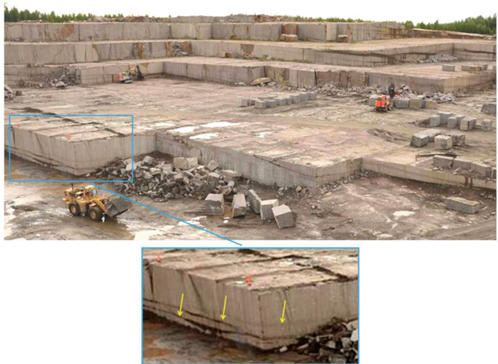
Fig. 1 General view of the modern pit of the Pyuterlakh granite deposit rapakivi (Finland). The arrows on the enlarged fragment indicate open cracks separately of different order. Photo by A. A. Zolotarev (2017)
