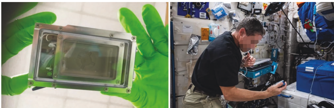
Fig. 10.21 View of one Rob2 hardware used onboard of the ISS (left) and Astronauts checking the correct rehydration of A. vaga individuals. Sixteen pieces of hardware were sent to ISS, each containing 40,000
