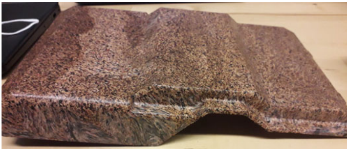
Fig. 4 Sample produced by compression molding of blend 2
