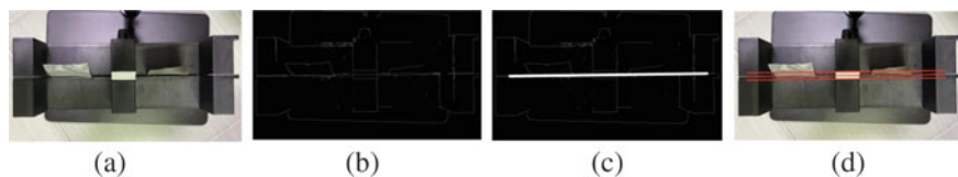
Fig. 5 Canny edge detection process: (a) input image, (b) result of Canny edge detection, (c) drawing the center line, (d) drawing the control line
