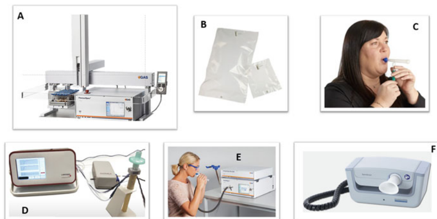
Fig. 4 Commonly used with IMS sampling devices: (a) FlavourSpec ® (G.A.S/ImSpex), (b) polymer bags, (c) Haldane sampler, (d) Loccioni ® sampler with CO 2 monitor, (e) direct online sampling, (f) SpiroScout ® (B&S Analytics)
