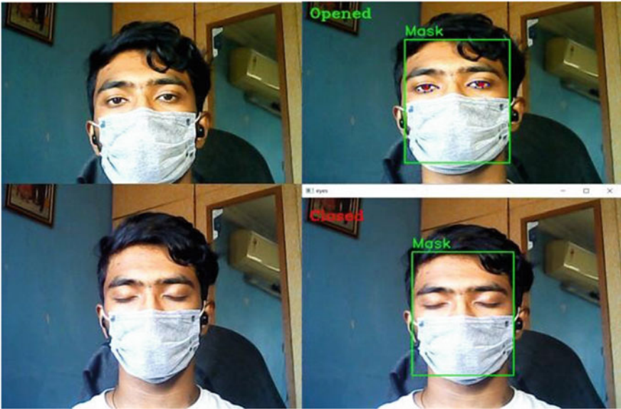
Fig. 8 Using webcam and Rpi to get input image for masked image
