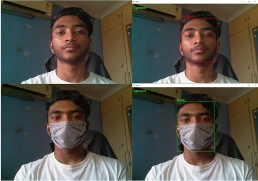
Fig. 7 Using a raspberry pi camera to get input image for masked and unmasked image
