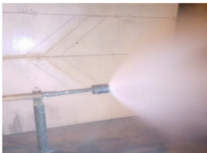
Fig. 4. Water atomization with a cone angle of 90^\circ
