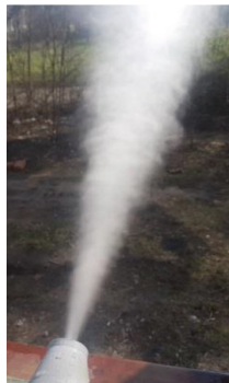
Fig. 2. Model liquid atomization with a pneumo-hydrovortex nozzle made by 3D printing
