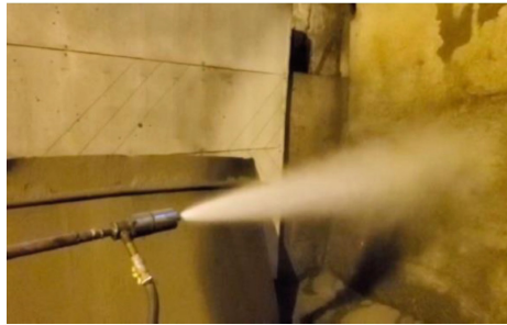
Fig. 3. Water atomization with a cone angle of 20°
