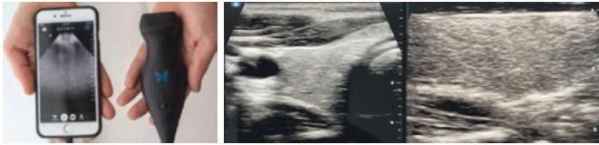
Image 1.2 Butterfly point-of-care system (left), an image displayed on an iPhone, with examples of transverse (middle panel) and sagittal (right panel) images of the thyroid
