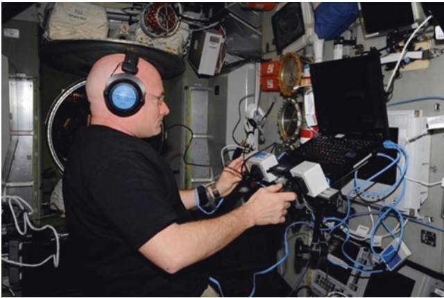
Fig. 4.2 Astronaut Scott Kelly using the 6df docking assessment platform during the joint US–Russian 1-year mission on board the ISS. Credit: NASA/RKA
