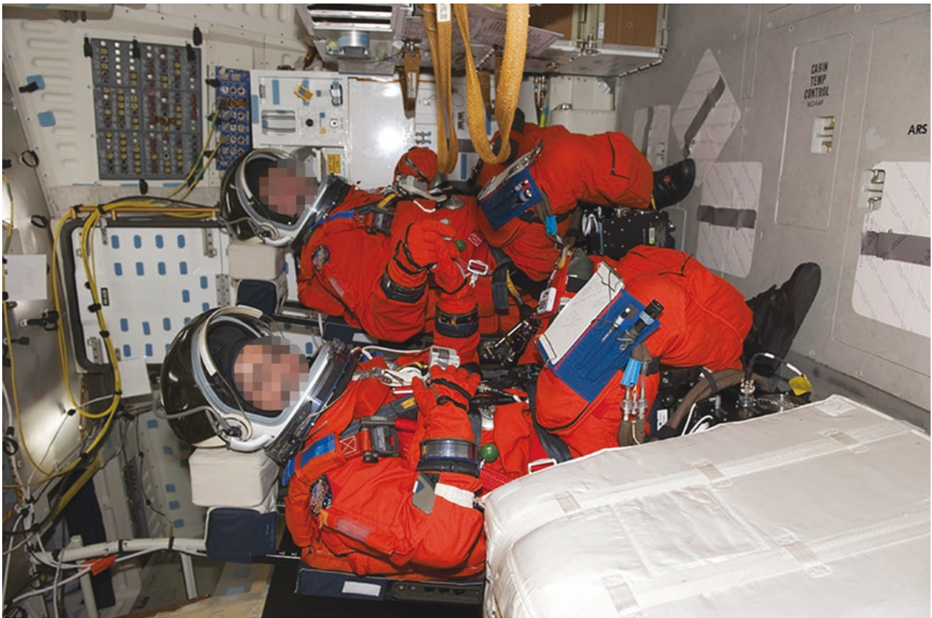
Fig. 2.3 The supine legs up posture is very common for launches (courtesy of NASA)
