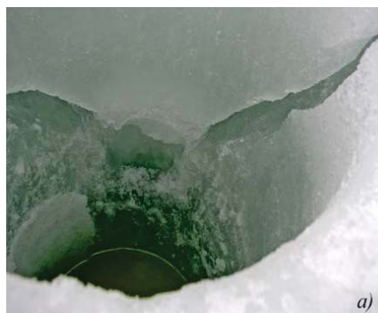
Fig. 9.8 Example of indenter penetration into the borehole side with ice chipping towards its surface: a ) - imprint from indenter in the borehole side and crack of ice chipping (view from aside); b ) - imprint from indenter and chipping of the surface ice part (view from above).
