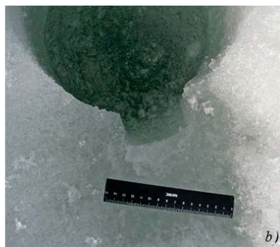
Fig. 9.8 Example of indenter penetration into the borehole side with ice chipping towards its surface: a ) - imprint from indenter in the borehole side and crack of ice chipping (view from aside); b ) - imprint from indenter and chipping of the surface ice part (view from above).
