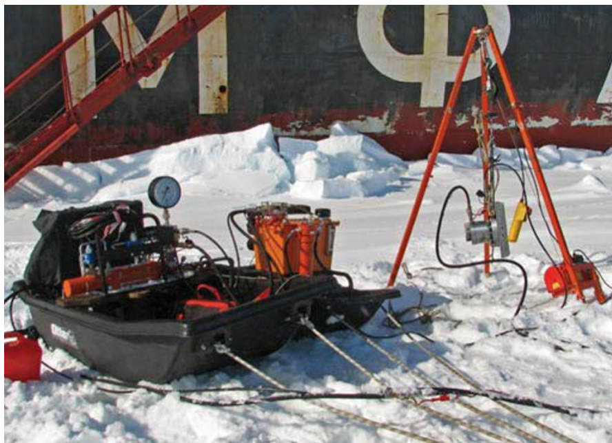
Fig. 9.5 Complex system for determination of ice strength characteristics in boreholes under the full-scale conditions.
