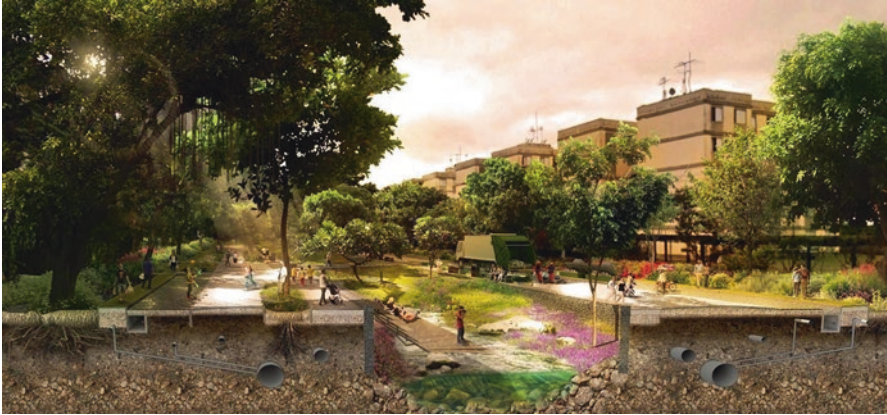
Fig. 4.5 The channels of the creeks can be revitalized by including additional proposed vegetation and re-designing the stream's land forms to manage current and future stormwater FCTH (2017)
