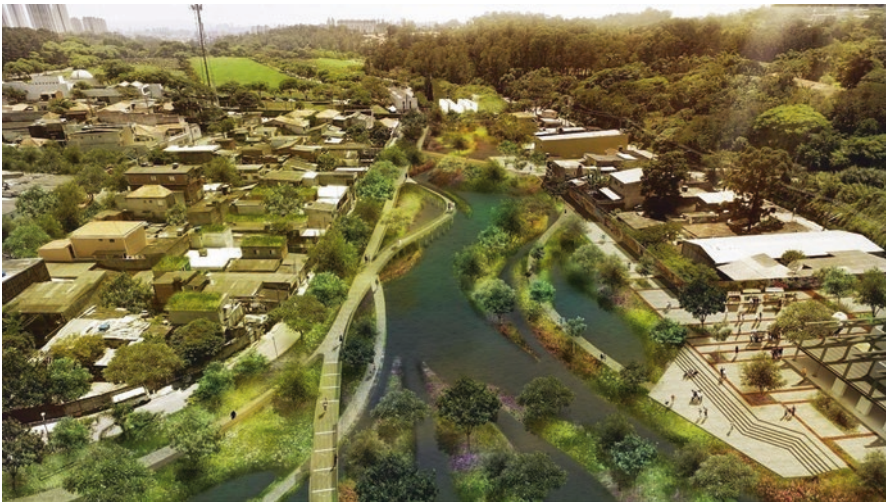
Fig. 4.6 A parametric process of design can give new dimensions to the detention ponds, as here where the green infrastructure overlays many functions FCTH (2017)
