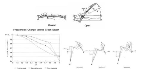
Fig. 15 Cross-section of a BS60CC 29 mm tilting-disk valve in the closed and open position, inlet strut frequency ratio changes for various crack depths of the left strut leg, and the first three modes of vibration change for varying crack-depth
