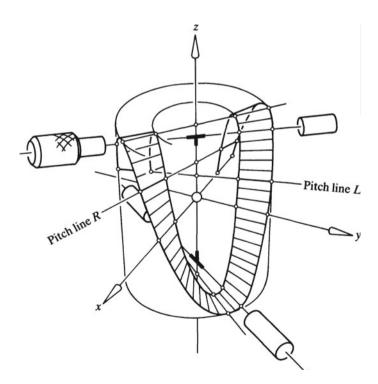
Fig. 3 The cylindroid generated by a spatial gear set
