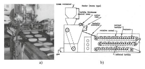
**Fig. 16** The automatic machine for production of Mexican tortillas investigated by Prof. López-Cajún with results in Figueroa et al. (2000): **a** the sample of the investigate machine; **b** a scheme of the historical-technical analysis
