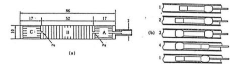
Fig. 8 In-pipe traveling micromechanism composed of three air balloons
