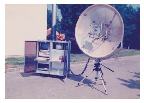
Fig. 14 The developed sound source exploration device with a parabolic sound collector and a microphone array
