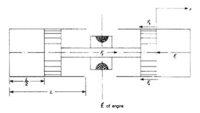
Fig. 17 Principle of the EIC engine operation
