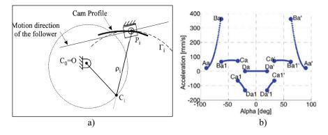
Fig. 14 An illustrative example of kinematic analysis of the circular-arc cam transmission (Carbone et al. 2001; Lanni et al. 2006): **a** identification of equivalent slider-crank mechanism; **b** results of the kinematic analysis in term of point acceleration
