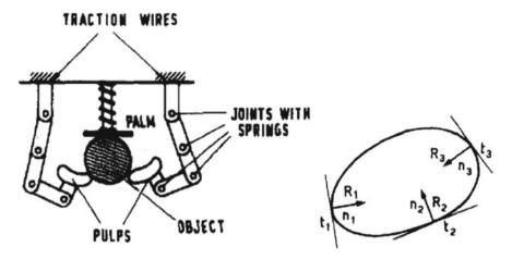
Fig. 12 Schemes for a robotic hand with multiple contact grasp by Bianchi and Rovetta (1978), Rovetta (1979, 1981, 1985)
