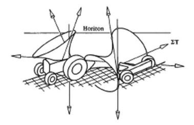
Fig. 2 Two sets of four balanced forces on the tractor and the trailed disc plough
