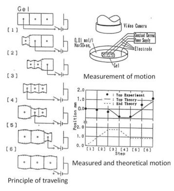
Fig. 11 Micro caterpillar made of high water absorbent electrolytic polymer-gel
