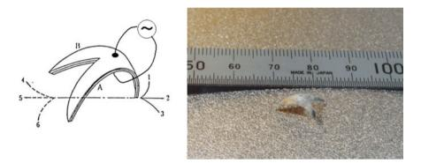
Fig. 9 Surface traveling micromechanism composed of piezoelectric film bimorph
