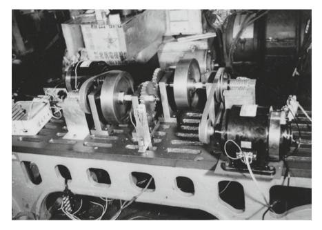
Fig. 5 The developed dynamic gear meshing tester
