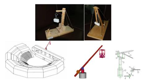
Fig. 9 Reconstruction of ancient lifting devices of the fifth century BC. From left, the monokolos, the dikolos, and below the Deus-Ex-Machina reconstruction in 1993
