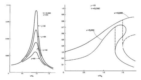
Fig. 18 Vibration spectrum of the EIC engine, left: low nonlinearity, right; high nonlinearity
