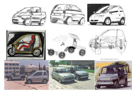
Fig. 21 Stylist's Dimitri Spanos, free-hand sketches of the mini city car Rio in 1990, the 3D model, the testing prototype and the car body model
