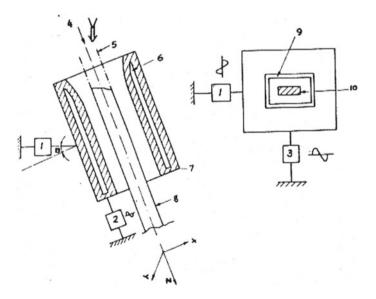
Fig. 16 Two cross-sections of a mold vibrating in the two lateral directions and the direction of longitudinal motion of the cast strand
