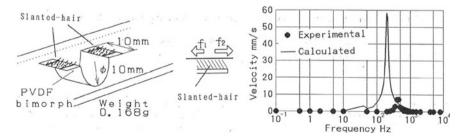
Fig. 10 Ceiling traveling micromechanism and its velocity
