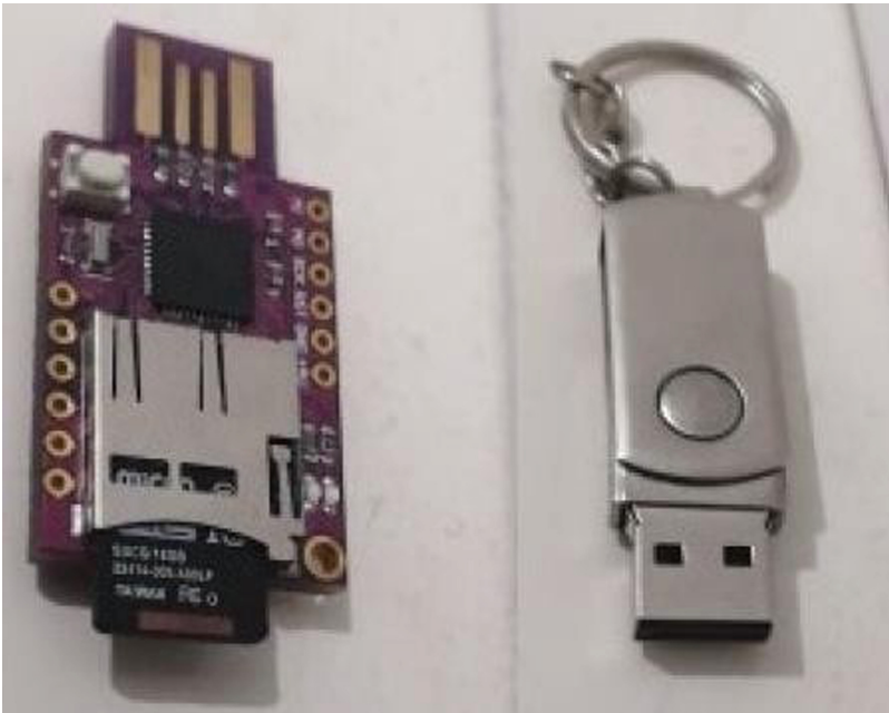
Fig. 3. BAD USB sticks (Left: Using a micro-SD card, Right: Without an external card).
