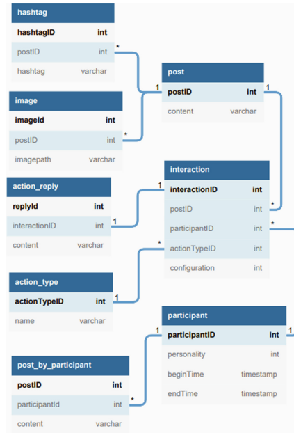
Fig. 4. Partial data model of the tables related to the prototype environment in First Normal Form
