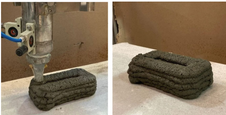
Fig. 7.7 Printing trial of the composition with 15% of SCBA
