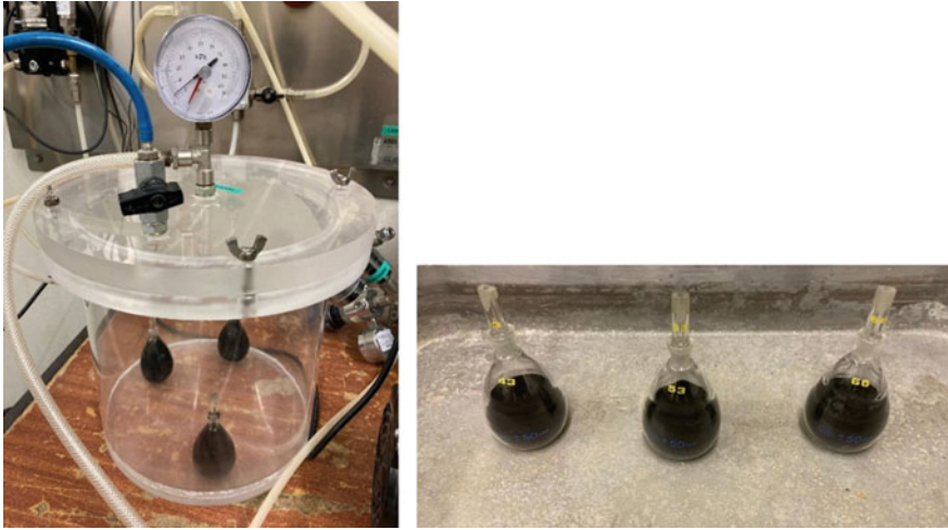
Fig. 7.2 Determination of SCBA’s bulk density with pycnometers
