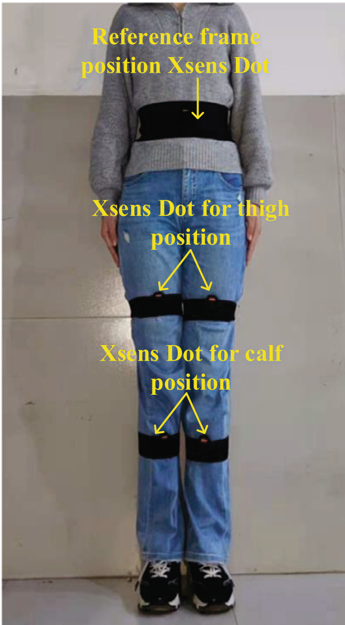
Fig. 4. Experimental equipment and target personnel.
