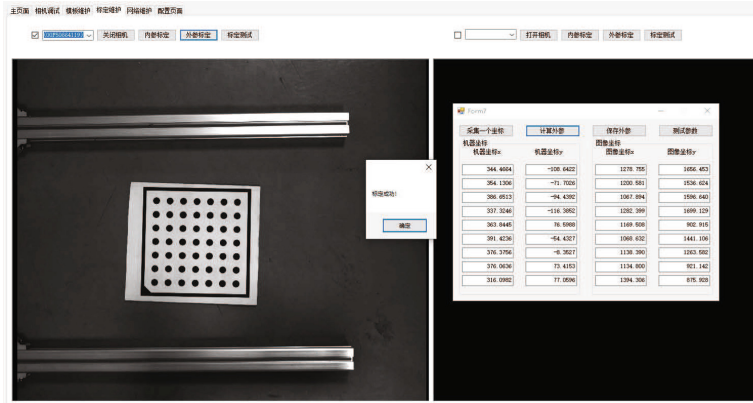
Fig. 5. The software completes the calibration of the camera.
