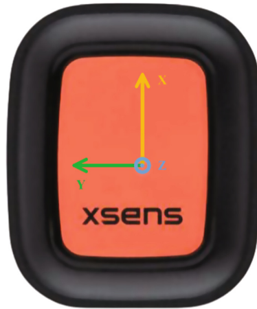
Fig. 2. Sensor coordinate system.
