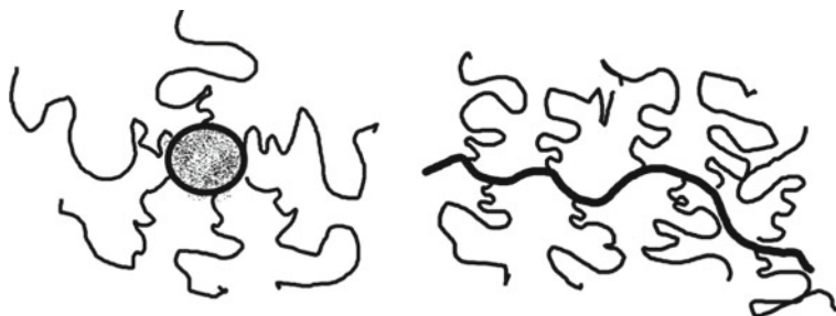
Fig. 21.1 Schematic representation of nonionic and ionic grafted copolymers
