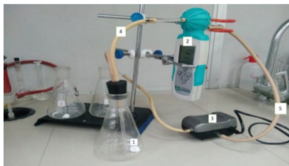
Fig. 2 Laboratory unit for measuring the diffusion of free formaldehyde: 1-conical flask with a sample of UFR or UFF, 2-flow gas analyzer for formaldehyde MIS-98170, 3-air compressor for air supply with two tubes, 4-tube that blows air with \text{CH}_2\text{O} with flasks and feeds in MIS-98170; 5-tube that absorbs air together with \text{CH}_2\text{O} from MIS-98170 and feeds into the air compressor
