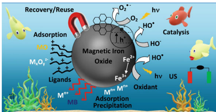
Fig. 6 Mechanisms of pollutants removal by magnetic iron oxide [51]
