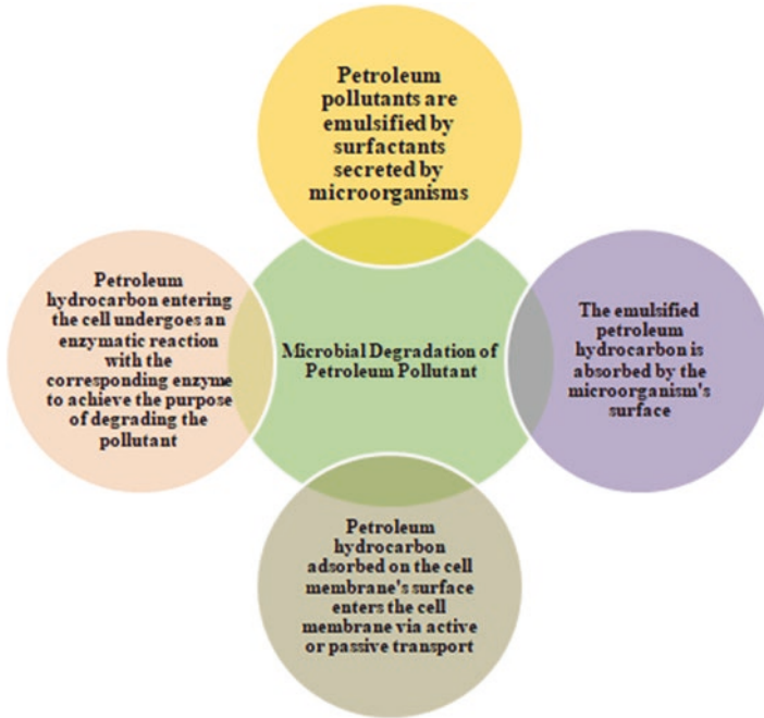
Fig. 8 Schematic diagram of four main phases of microbial degradation of petroleum hydrocarbons
