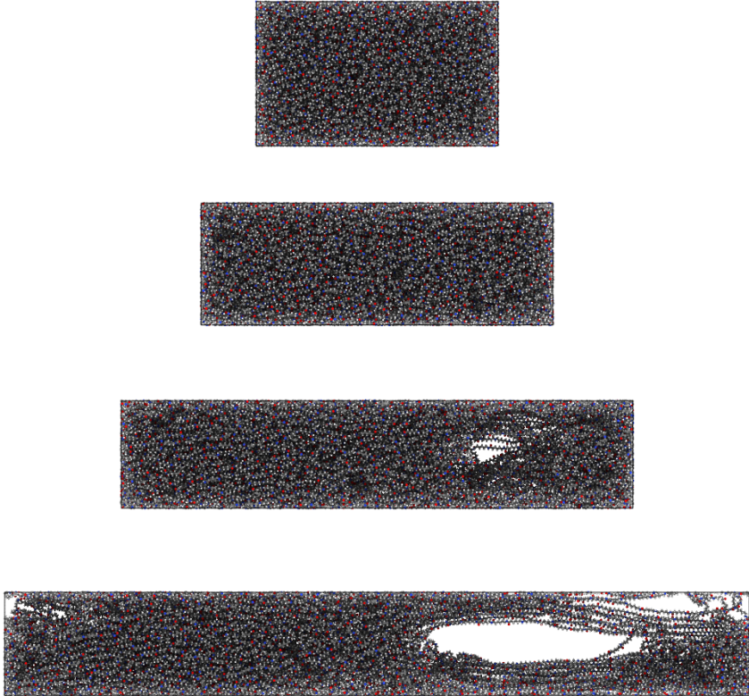
Fig. 6: Simulated tensile test for dry PA6 with lateral contraction for a true strain rate of 1.0 \times 10^{-6} 1/fs after 25, 50 and 100 % simulation time and 45.5 %, 111.7 %, 208.0 % and 348.2 % strain respectively. The color coding is the same as before (H: White, C: Grey, N: Blue, O: Red). Visualization with Ovito [8].
