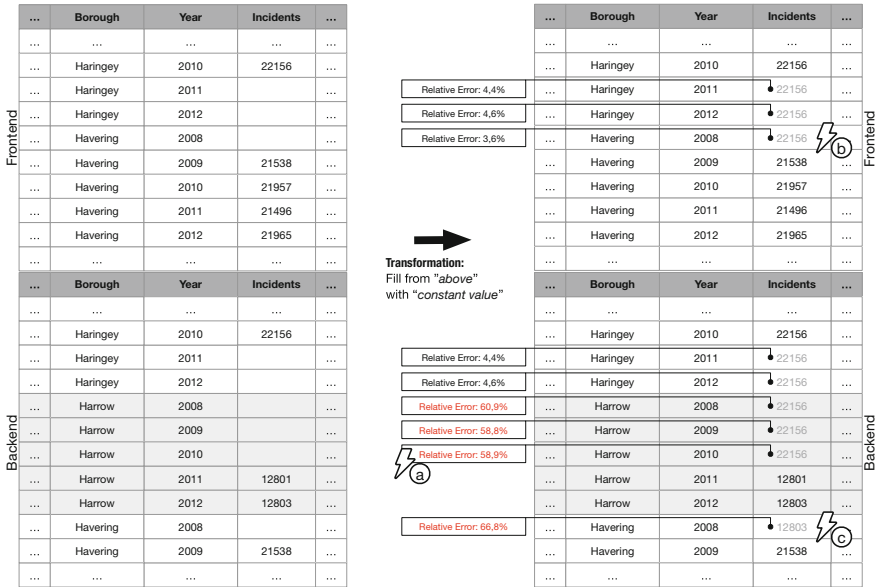
Fig. 1. Discrepancy between perceived state in the frontend and the actual state in the backend applying a “Fill”-transformation to impute missing values. Gray shaded rows indicate data only contained in the backend, thus unperceived by a domain expert.
