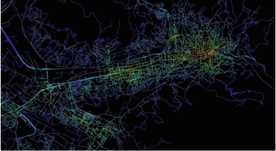
Fig. 4. Global Integration R1200. Illustration depicts most integrated city areas for 15-min pedestrian movement
