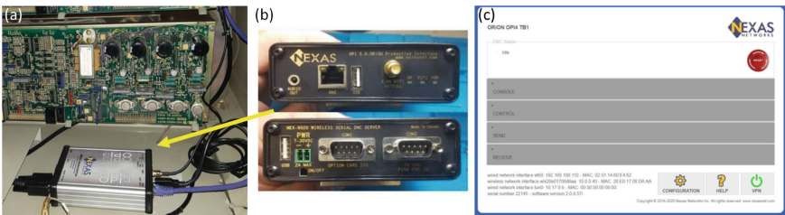
Fig. 1. (a) Nexas ORiON Production Interface (OPI) installed in CNC machines. (b) Front and back view of the OPI. (c) Web interface of the OPI.
