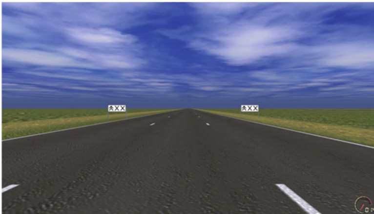
Fig. 1. Screen shot of the Lane Change Test (LCT) with road sign instructing move to left lane
