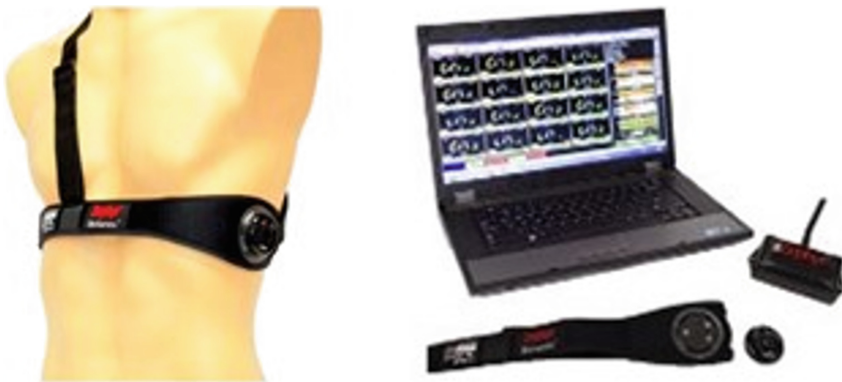
Fig. 2. Bioharness telemetry & logging system (from Bioharness manual book)
